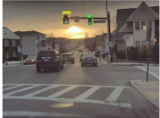
Fig. 4. YOLOv3 traffic light detection
