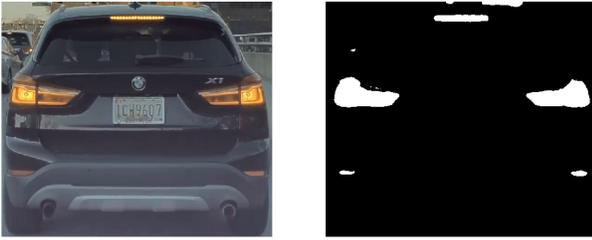
Fig. 14. Brake lights detection using YCbCr thresholding
